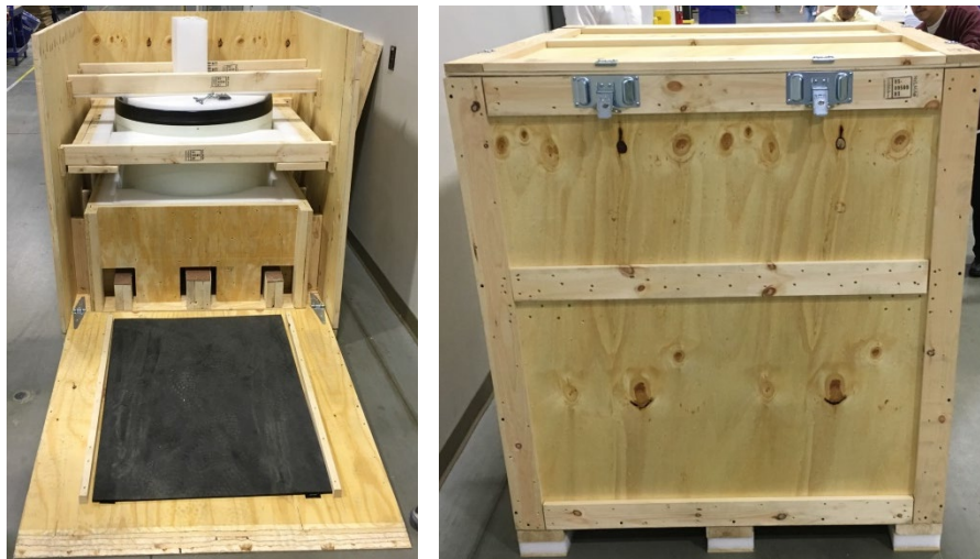
Figure 29. OPUS 80R Pre-packed Chromatography Column shipping container design
