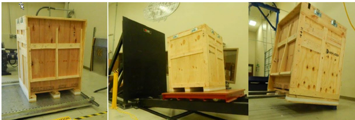
Figure 30. OPUS 60R Pre-packed Chromatography Column vibrational, incline impact, drop testing
