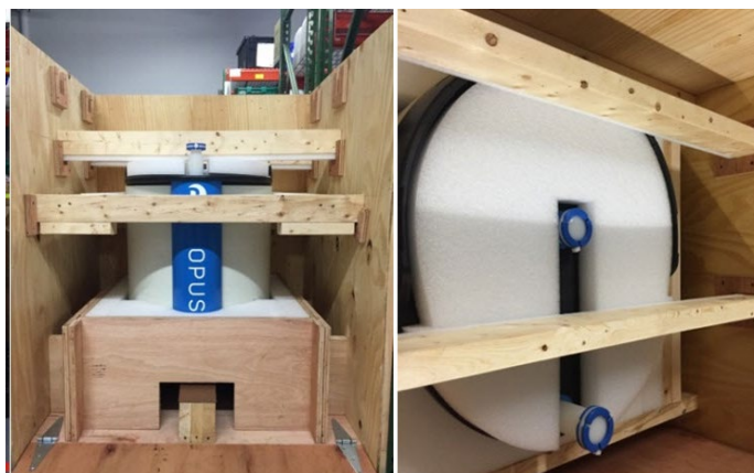
Figure 27. OPUS 45R and 60R Pre-packed Chromatography Column shipping container design
