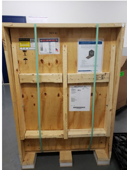
Figure 29. OPUS 80R Pre-packed Chromatography Column shipping container design
