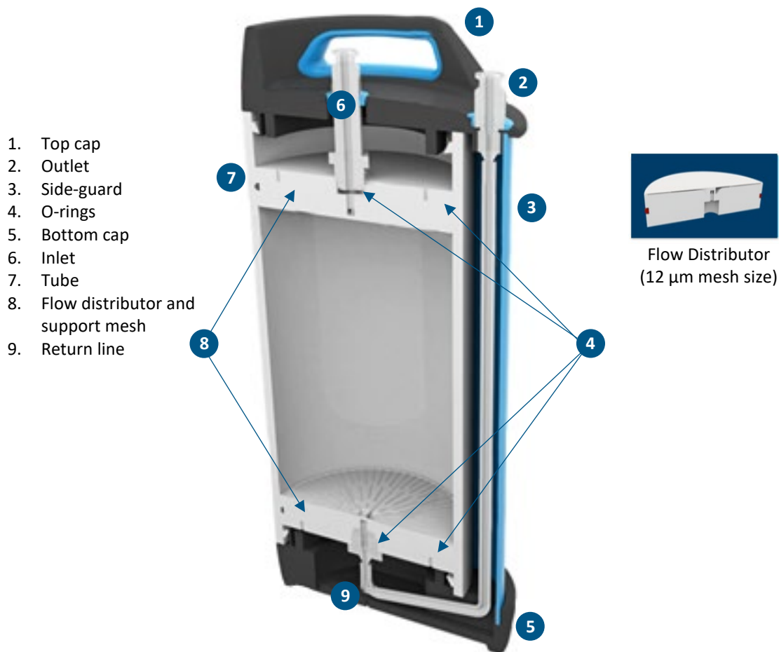
Figure 8. OPUS 10 – 30 Pre-packed Chromatography Column design (OPUS 20 shown)
